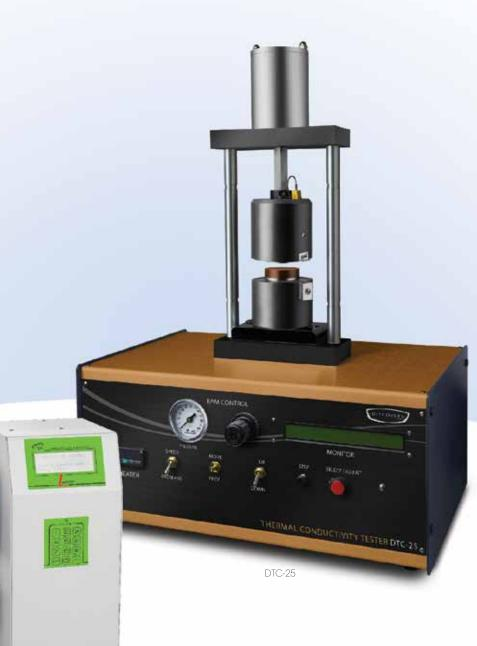
The most intuitive solution for testing insulating materials in accordance with international standard test methods ASTM C177, ISO 8302, and EN 12667
