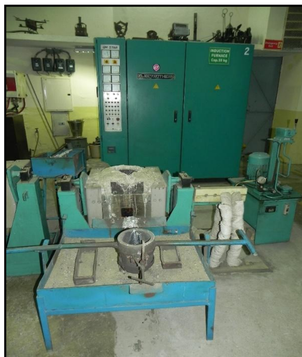
Fig. 5: Furnace for melting metal for pouring into mold.
