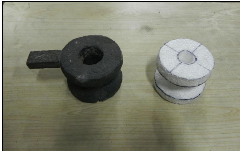
Fig. 3: Foam pattern and the corresponding cast object.
