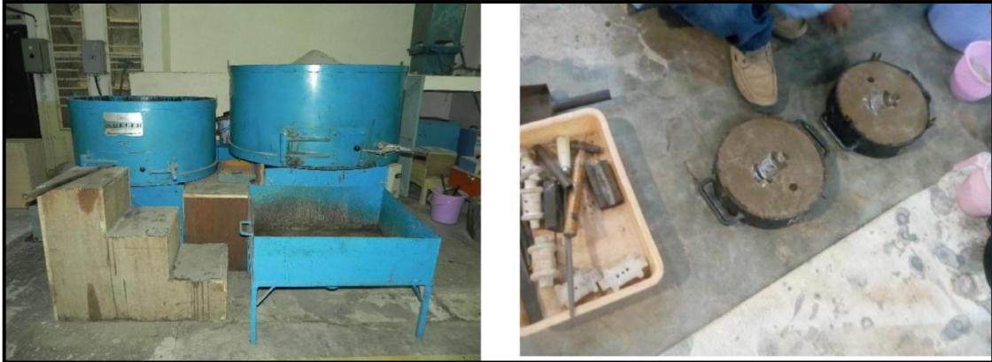
Fig. 4: Equipment for sand mixing and a prepared mold.
