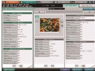
Job ticket editing screen Change detailed output settings including paper type and number of copies.
