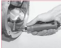
Finishing a casted workpiece with the 12S1000-36
