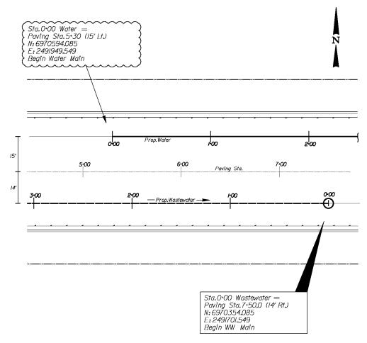
FIGURE 2.9: STATIONING CONVENTION AND CROSS-REFERENCING
