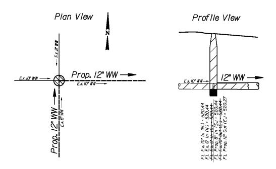
FIGURE 2.14: FLOWLINE CONFIGURATIONS AT WASTEWATER MANHOLE
