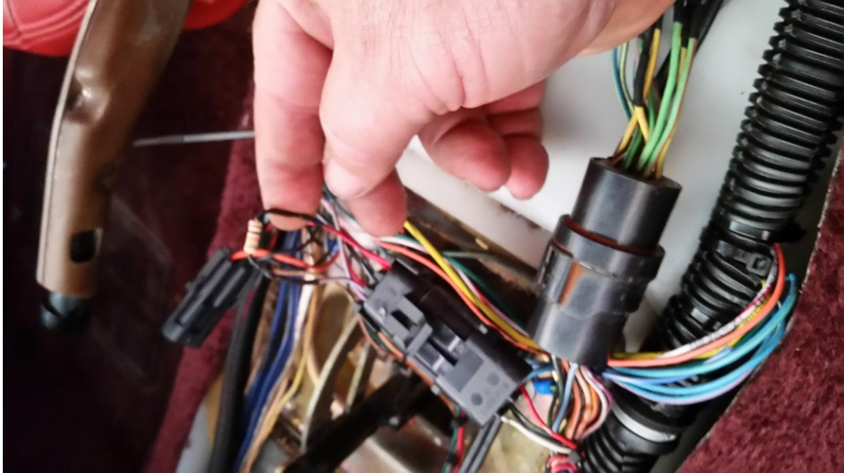
Figure 4 - Wiring in a Pull-Up Resistor in to the VSS Plug
