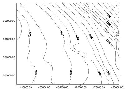
The bedrock topography is shown below from a SURFER file called bedrock.grd. The bedrock elevations range from 431 ft msl to 1104 ft msl.
