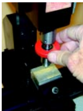
FIG. 105 —The chuck is lowered using the collar.
