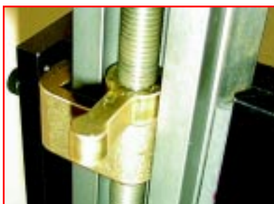
FIGURE 58—The saddle locking lever provides a positive lock for the Z-axis and is standard on all new (non-CNC-ready) Sherline mills.
