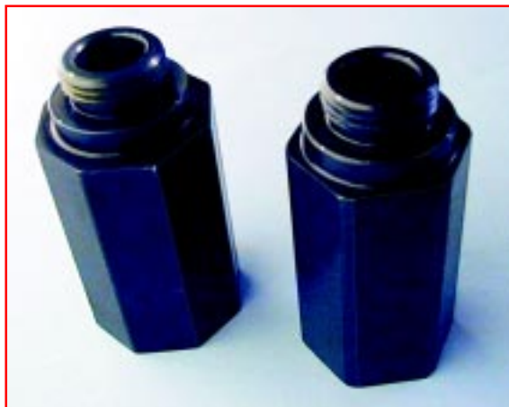
FIGURE 82 —An indexing set offers an easy way to index simple hole patterns or do milling on 2, 3, 4, 6 or 8 sides.
