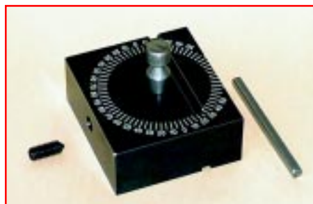
FIGURE 100— Mill headstock spacer block, precision-ground alignment key and set screw
