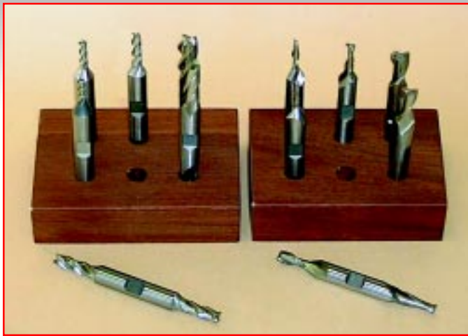
FIGURE 71 —Double-ended 3/8" end mills fit in the P/N 3079 end mill holder. They are available in a large variety of sizes and shapes. For strength and maximum rigidity, use the largest diameter cutter your job will allow.
