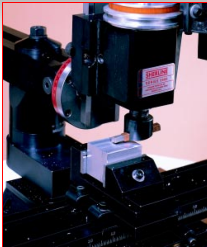
FIGURE 97 —Fly cutting is an excellent way of producing a flat surface quickly. This Model 5400 mill has been converted to 8-direction capacity with a P/N 5650 column upgrade. The adapter base can be seen in the background.
