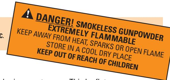
Smokeless powder does not detonate like high explosives as it has a controlled rate of burn and differs considerably in its burning characteristics from common "black powder." Black powder burns at essentially the same rate out in the open (unconfined) as when in a gun.
