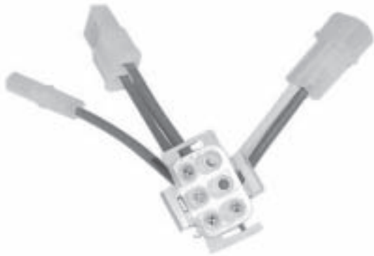
611296 - Converts new style 6-pin connector to the older 3 Amp. D.C., 5 Amp A.C. (3/5), 2-pin connector.
