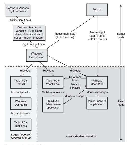
**Figure 4-1** The Tablet PC tablet input subsystem architecture, shown running on Windows XP Tablet PC Edition
