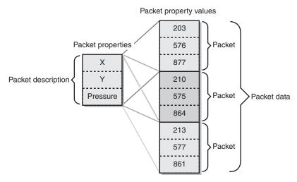
**Figure 4-8** The relationship of packets, packet properties, packet property values, and packet description
