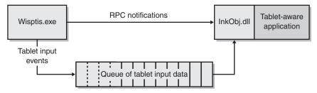
**Figure 4-4** Wisptis.exe communicates tablet input data to a tabletaware application through a queue to avoid losing any data.
