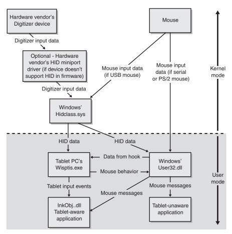
**Figure 4-2** The Tablet PC tablet input subsystem architecture, shown running as the Tablet PC runtime libraries on a Windows-based operating system
