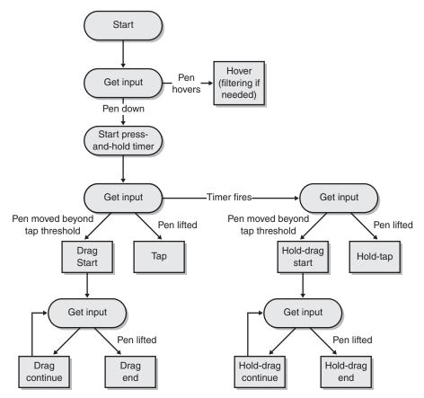
**Figure 4-3** A high-level state diagram illustrating how pen-based actions are detected
