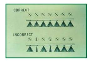
Streaking and puddling, two extremes of application, indicate improper spread rates or improper height of the spray bar.
