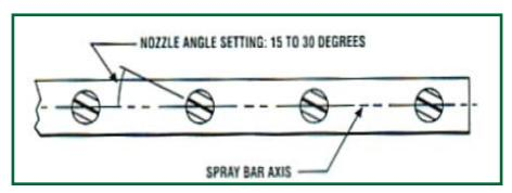
Set the spray bar nozzles at an angle between 15° and 30°.
