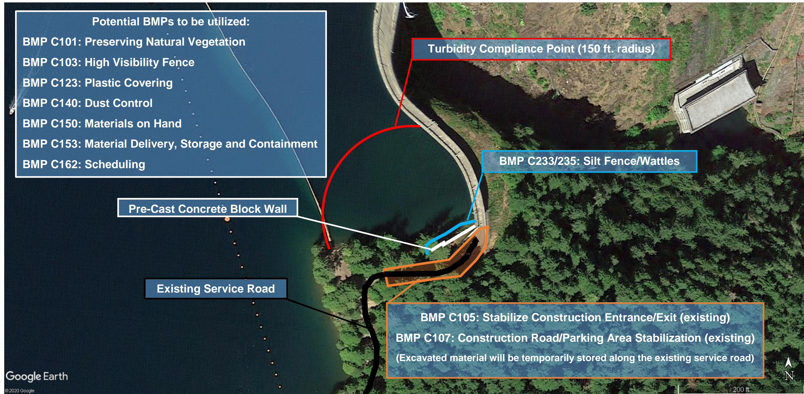
Figure 3. Cushman Dam #1 abutment and service road repair locations of actions, BMPs and compliance point.
