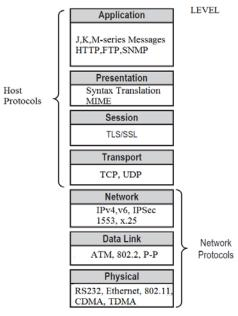
.Figure 3. The equivalent ISO OSI reference model [1]
