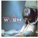
Monitor (WVSM)—a mobile device that allows medical personnel to be connected with multiple-patient monitoring data remotely and up to 20 patients simultaneously. The WVSM monitors, transmits to a PC or Apple device, and records four hours of BP, HR, SpO2, and 3-lead ECG patient trending data. The WVSM is FDA cleared.
