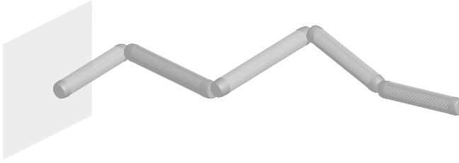
Fig. 10.4 Geometrically exact fixed-free elastic rod
