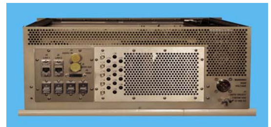
Figure 2. The rear panel includes all analog signal connections and can be customized to suit the application requirements.
