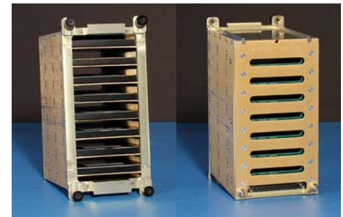
Figure 5. Front and rear view of the QuickPac canister showing the eight SSDs inside.
