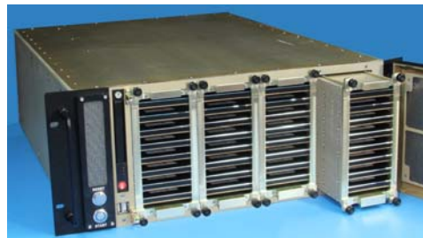
Figure 4. Chassis View showing one QuickPac canister partially withdrawn.
