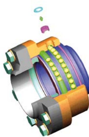
Swivel joint for petroleum products
