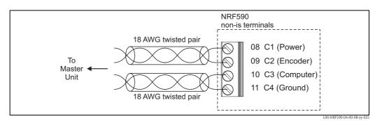
Fig. 1: Wiring diagram for L&J Tankway Protocol
