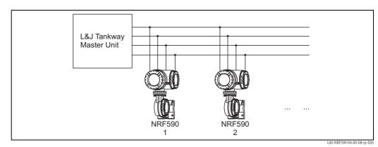
Fig. 2: Standard topology for L&J Tankway Protocol
