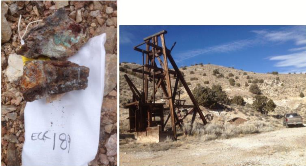
Silver Bear Prospect- Grab Sample from Mullock/Dump material & old headframe In northern part of prospect area. ECR189 – 14.6% Zn, 427 g/t Ag, 3.8% Pb, 0.4% Cu, 0.3 g/t Au
