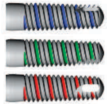
Fig. 1B Side view of implant with one thread colored to indicate the presence of three threads traversing the length of the threaded portion of the implant.
