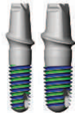
Fig. 3B 3.7mmD and 4.7mmD Zimmer One-Piece Implants have double-lead threads with a 0.6mm thread pitch. Similar to the 3.0mmD Implants, each complete turn will seat the implant 1.2mm.
