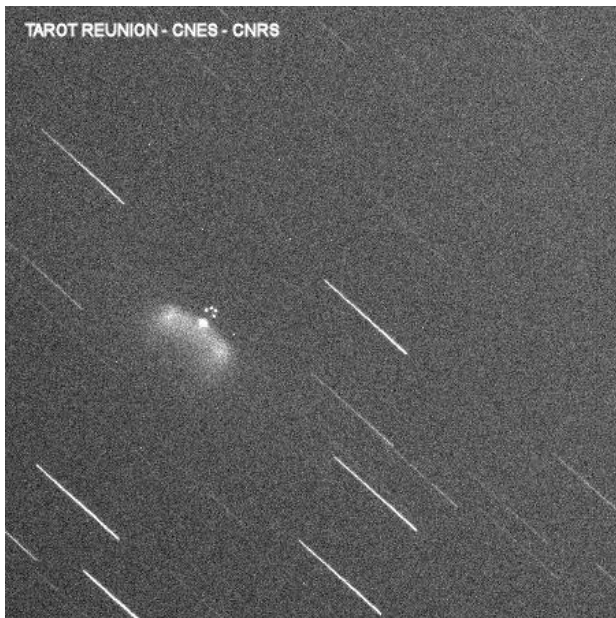
Figure 13: The Ariane V233 launch of four Galileo spacecrafts. The EPS is seen outgassing before passivation, and the four Galileo satellites are clearly seen and released by pairs (TRE image, CNRS – CNES).
