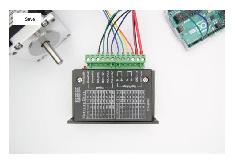
In this tutorial, you will learn how to control a stepper motor with the TB6600 microstepping driver and Arduino. This driver is easy to use and can control large stepper motors like a 3 A NEMA 23 (https://amzn.to/2HpVx6b).
