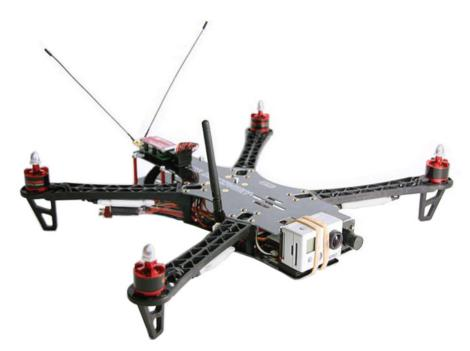
The TBS DISCOVERY comes as two main boards (top and bottom) and optional Flame Wheel arms with accessories. It transforms the popular F450 (Flame Wheel) into a spider quadrotor. The GoPro and FPV camera mount is placed ideally for "no-prop-in-view" pictures. The optional TBS CORE can be placed directly onto the frame or we can install it for you.
