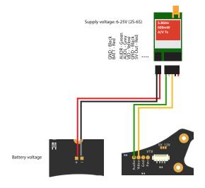
\$ On 4S+ setups where 12V is not available, consider using a dedicated TBS CORE PNP to supply power to the video transmitter.
