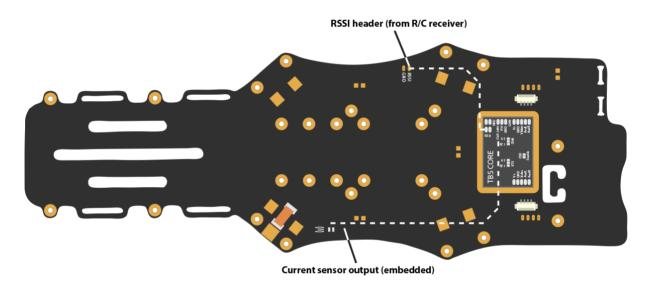
• Lastly, when all the R/C and FPV gear is installed, connect any the remaining R/C or RSSI cables to the top plate and close the frame. Use the remaining spacer and frame arm screws to secure the frame.
