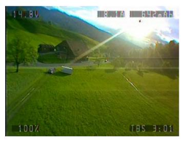
You can use an optional (but recommended) OSD add-on to get live readout on screen about the battery voltage (V), current draw (A), total current consumption (mAh), receiver signal strength (%) and flight time (minutes:seconds), position (coordinates) and home location, to name a few. For a basic feature set we recommend the TBS CORE which provide all but the latter two data points. A full feature set will require an OSD with a GPS module (e.g. TBS CORE PNP PRO with GPS).
