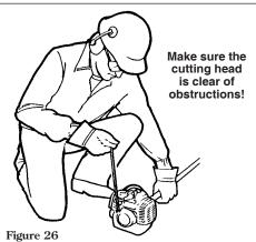
5. While holding the outer tube firmly with one hand, slowly pull the recoil starter handle until resistance is felt, then pull quickly to start the engine.
