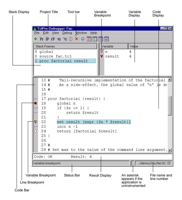
Figure 1 TclPro Debugger Main Window
