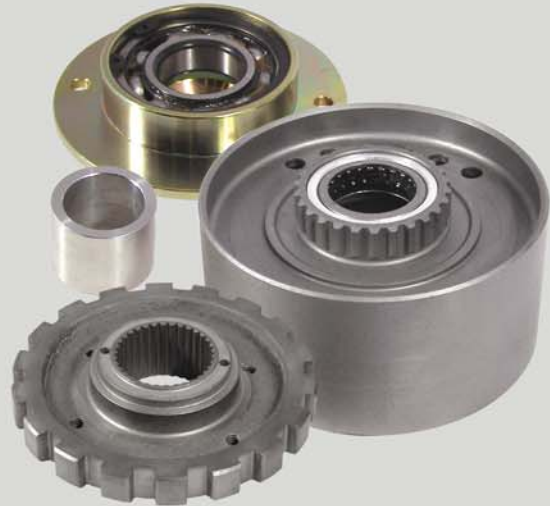
A727 Sportsman Support Kit: #K120005 TCS has modified the steel OEM low/reverse drum to incorporate a caged needle bearing to reduce drag and friction. Output support made from billet steel with large radial ball bearing. Lightened parking gear. Governor elimination sleeve. *Note: Use only with a manual valve body or transbrake valve body.
