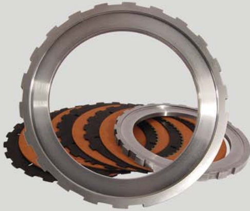
TH400 Center Support & Oversize Piston: #223704 For high power applications e.g. supercharged, turbocharged, nitrous and mega cubic inch engines. Piston and bore diameter increased 1/4" for more clamping force on the intermediate clutch pack.
