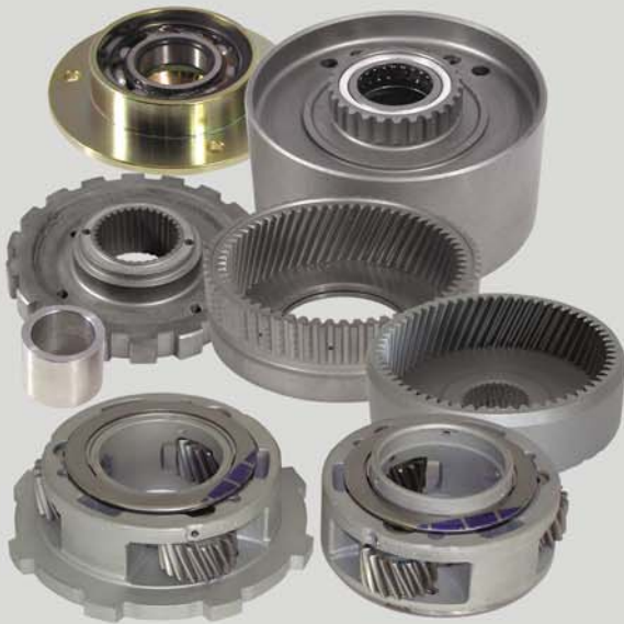
A727 4-Pinion Sportsman Planetary Assembly: #K127500B (75 & older) #K127500E (76-93) 4 enclosed Torrington needle bearing assemblies. New front planetary steel top-hat - for maximum spline strength. Radial ball bearing output support made from billet steel. Stock ratio 2.45/1:45. roller bearing installed in a refurbished O.E.M. 1st/reverse drum reduces friction. TCS governor elimination sleeve, plus lightened park gear. Available as a 4 pinion assembly. *Note: Use only with a manual valve body or transbrake valve body.
