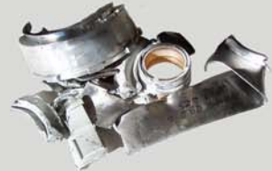
K123900AS 22,640 RPM equal to: 10,290 engine RPM FAILURE SPEED
