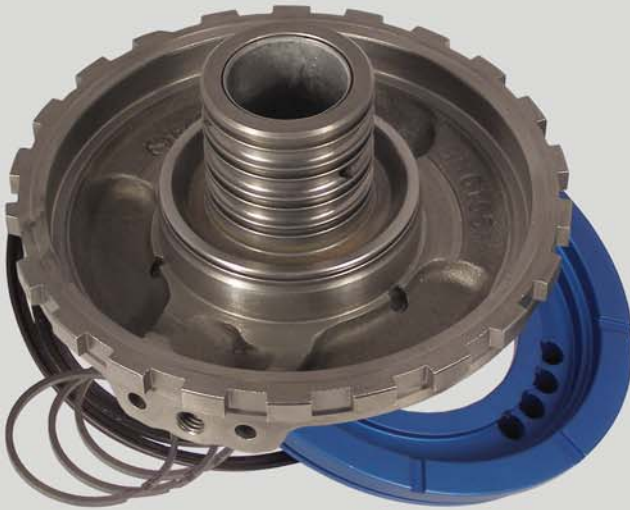
TH400 Center Support & Oversize Piston: #223704 For high power applications e.g. supercharged, turbocharged, nitrous and mega cubic inch engines. Piston and bore diameter increased 1/4" for more clamping force on the intermediate clutch pack.
