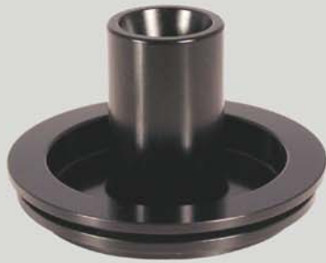
A727 Low/Reverse Aluminum Piston: #123003 Made from billet aluminum. Eliminates cracking failures common to the O.E.M. part in a transbrake application. Eliminates spring and messy shims.
