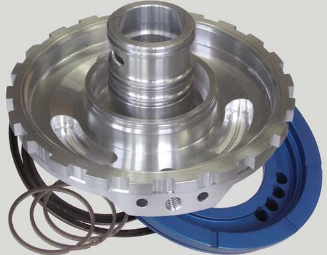
TH400 Aluminum Center Support & Oversize Piston: #223704A Billet aluminum support is for high performance applications. Much lighter than the OEM version. Piston and bore diameter increased 1/4" for more clamping force on the intermediate clutch pack.
