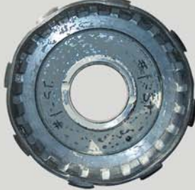
K123900S 25,000 RPM equal to: 11,363 engine RPM FAILURE SPEED
