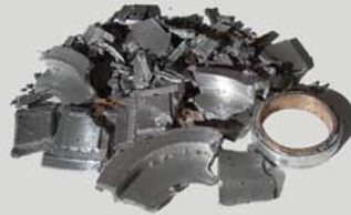
K123900 36,550 RPM equal to: 16,614 engine RPM FAILURE SPEED
