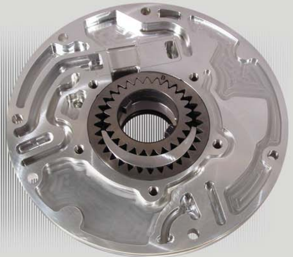
TH400 Aluminum Pump Body: #223400B The TCS billet aluminum 6061 body is 42% lighter than the OEM assembly. Bolts together with the OEM stator support. Added lubrication in gear area, Anti-spin features in front bushing area and snap ring retains front seal. "NO Blowout". 100% drop-in assembly.
