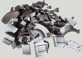
OEM 14,000 RPM equal to: 6,300 engine RPM FAILURE SPEED
