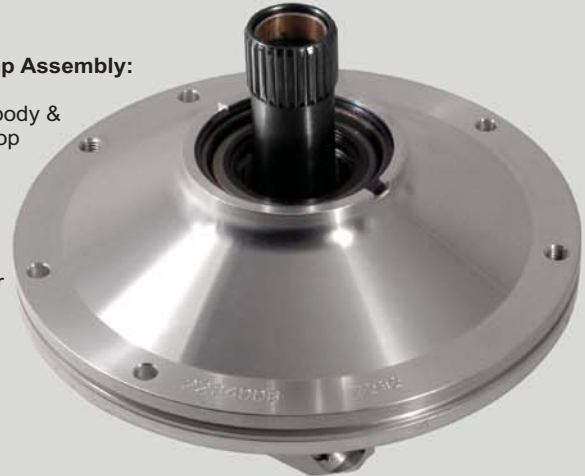
TH400 Aluminum Center Support & Oversize Piston: #223704A Billet aluminum support is for high performance applications. Much lighter than the OEM version. Piston and bore diameter increased 1/4" for more clamping force on the intermediate clutch pack.
