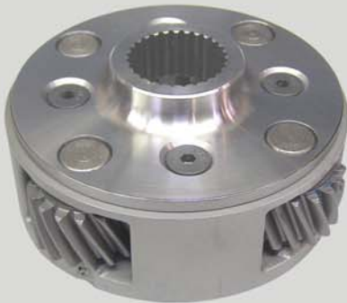
A727 4-Pinion Front Planet Assembly: #1275-1-BW (1975 & older) or #1275-1-EW (1976-93) This is a direct replacement front planet assembly that has been manufactured with a steel spline instead of aluminum as in the OEM version. The unit uses the OEM thrust washer for easy installation.
