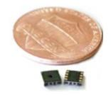
Ultrasonic time-of-flight distance measuring sensors
