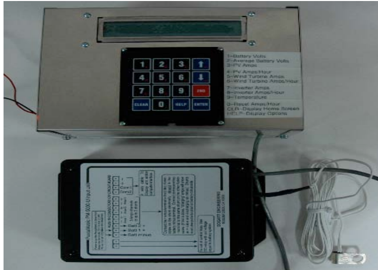
Figure 7: Data Logging System.
