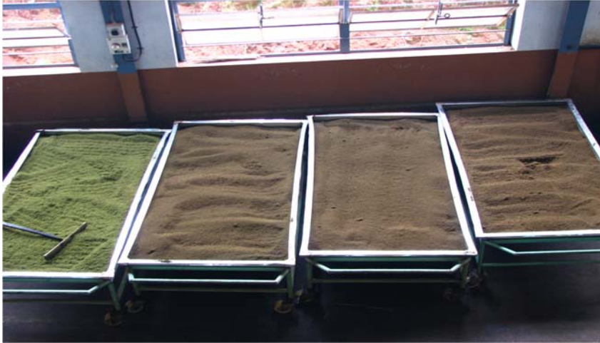
Fig 36: Oxidation process during the manufacture of black tea
