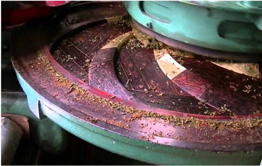
Fig 35: Maceration process using orthodox machine
