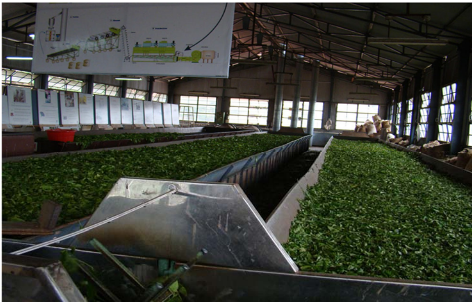
Fig 34: Withering of green leaf under in a factory on withering units with fans
