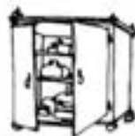
15. cabinet doors not fastened
