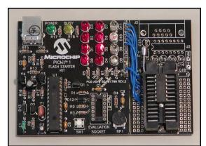
Figure 3. Modified PICKit1 Development Board
