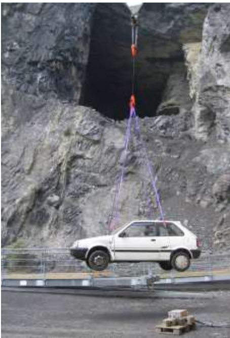
Picture 5.4 A high-tensile steel wire ( 1'770 \text{ N/mm}^2 ) with a diameter of only 3.0 mm is lifting a car 8
