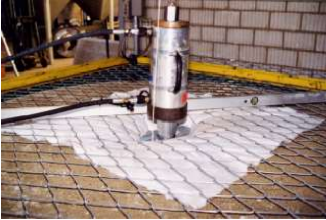
Picture 7.1 Test setup for puncturing test with TECCO® spike plate
