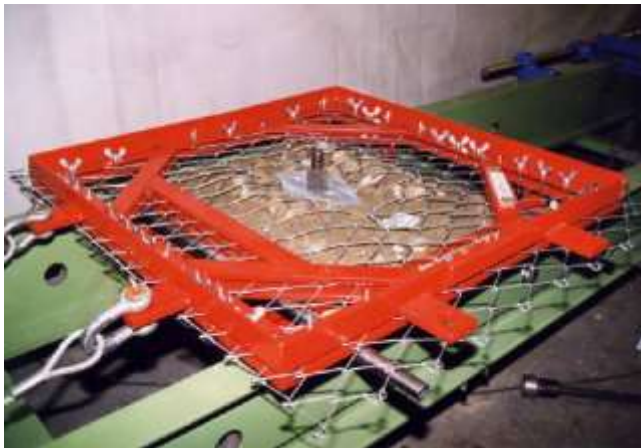
Picture 6.1 Test unit for determination of tangential force transmission test
