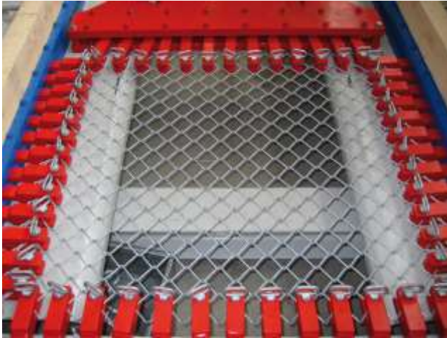
Picture 5.31 Test setup for the comparison tests with made from normal steel wires (550 – 650 N/mm 2 )
