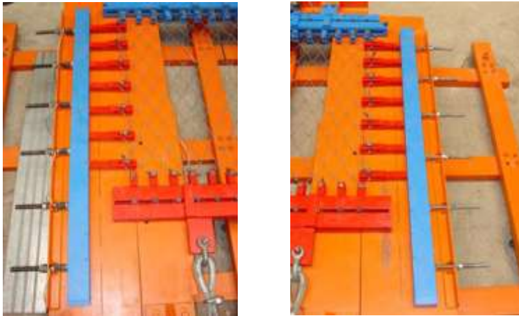
Pictures 5.9 Lateral fixation system of sliding beams to adjust the width of the test sample. In the left the connecting screw bolts that serves as transversal load measurement devices.
