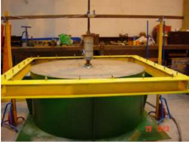
Picture 7.2 Puncture test with spike plate only (without any mesh)
