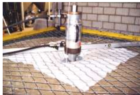
Picture 9.2 Test setup to investigate the puncturing resistance
