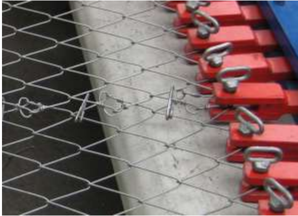
Picture 5.25 Detail of test arrangement for clip tests
