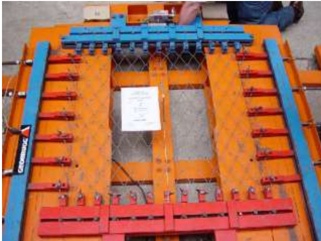
Picture 5.13 Experimental setup for tensile tests in the longitudinal direction
