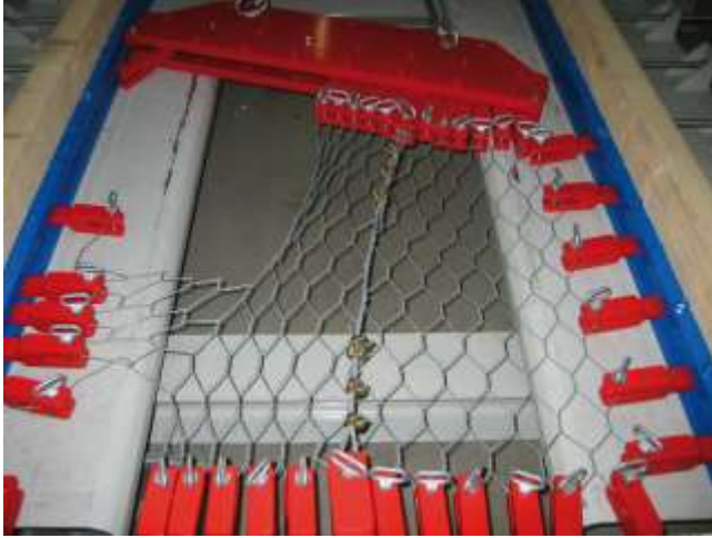
Picture 5.35 The steel wire rope does not significantly support the hexagonal wire mesh because the wire rope can only transfer load if it is fully straight. As long as the steel wire rope is curved (e.g. "S-form"), it is unable to transmit tensile forces in order to support the loads that are applied to the hexagonal steel wire mesh
