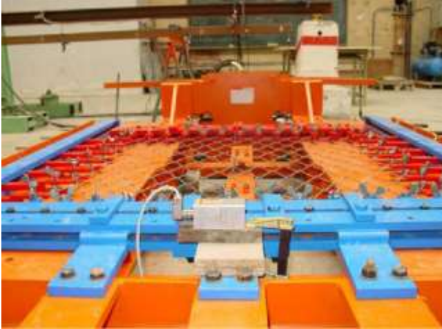
Picture 5.11 Detail of the device for the measurement of the longitudinal deformation
