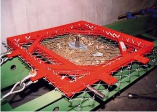
Picture F.1 Test setup to determine the bearing resistance of the high-tensile steel wire mesh system against selective, slope-parallel tensile stress. In this test series, the tensile forces have to be transmitted from the pulling machine, via wire ropes and shackles, the steel frame and the steel wire mesh onto the spike plate as well as the nail into the subsoil. The box filled up with sandy gravel and the central arranged nail with the spike plate are fix. The red frame and the attached steel wire mesh TECCO® can move freely on the green steel profiles
