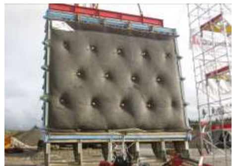
Picture 13.4 Test no. 5, TECCO® G65/3 + P33 = 85^\circ sandy gravel 0 – 63 mm
