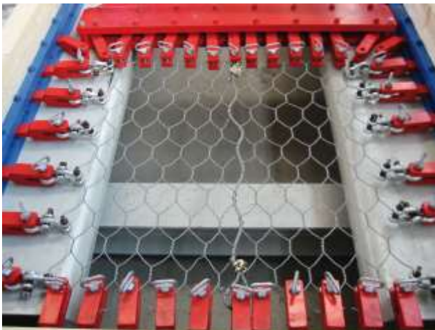
Picture 5.34 Test setup for the comparison tests with the reinforced hexagonal made from normal steel wires (approx. 350 - 550 \text{ N/mm}^2 ); reinforcement by 8.0 mm steel wire rope (centrally arranged)
