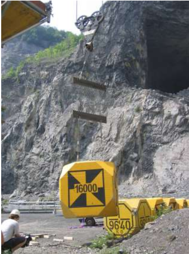
Picture 5.5 A concrete block with the weight of 16 metric tons (16'000 kg) is lifted up by a small stripe of a high-tensile steel wire mesh with wire diameter of 3.0 mm 9
