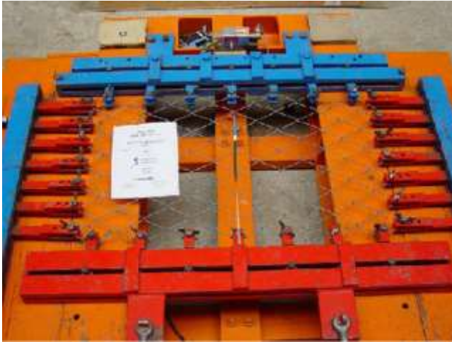
Picture 5.14 Experimental setup for tensile tests in the transverse direction
