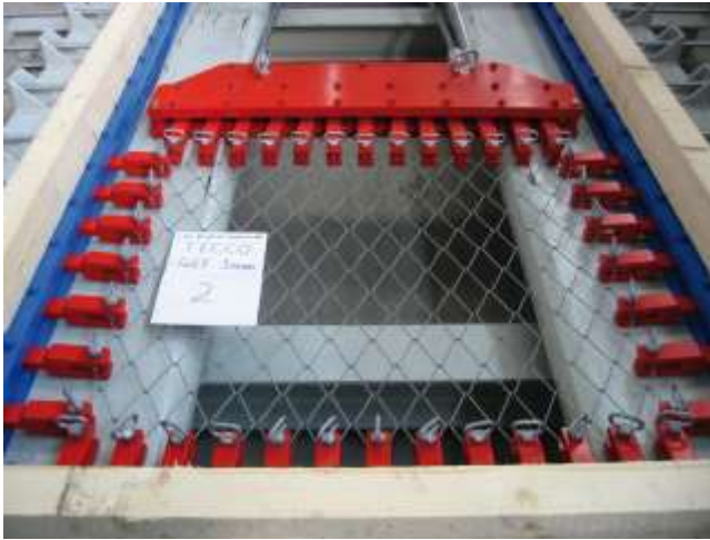
Picture 5.33 Test setup for the comparison tests with mesh made from high-tensile wires ( 1'770 \text{ N/mm}^2 )
