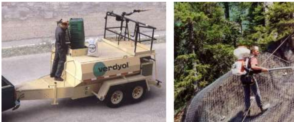
Picture 10.19 Left: Example for hydraulic seeding machine Right: Greening backpack (hand machine) for dry seeding
