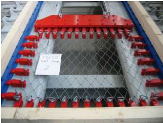
Picture 5.30 Test setup for the comparison tests with mesh made from high-tensile wires (1'770 N/mm 2 )
