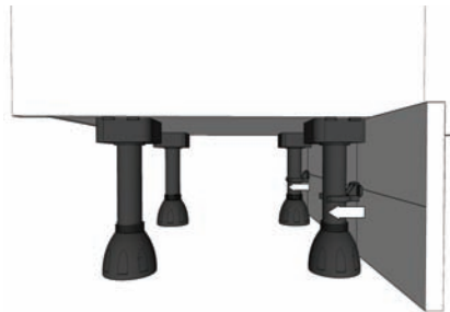
5 Screw the plinth clip back plate central to the markings made in the last step. Then slide the plinth clips onto the back plates. Finally offer the plinth with the clips into place and slide the clips onto the back plates to line up with the legs before pushing the plinth into place allowing the clips to spring around the legs
