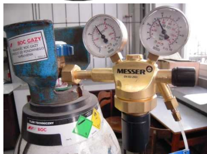
Figure 8. Pressure reducer valve with manometers, mounted to pressure gas can with O 2 .
