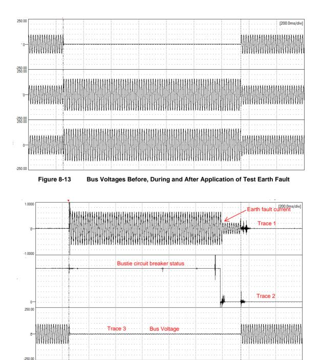
Figure 8-14 Earth Fault Current, Bustie Status and Bus Voltage
