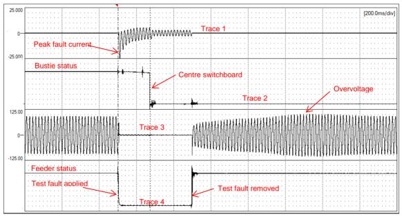
Figure 8-9 Fault Current, Bus Voltage and Status for Bustie Circuit Breaker and Feeder Circuit Breaker
