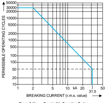
Figure 8-11 Permissible Operating Cycles
