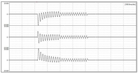
Figure 8-7 Measured Short Circuit Current at Feeder to Test Fault
