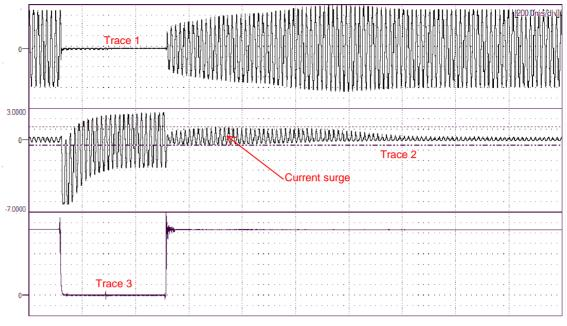
Figure 8-10Generator Current During Fault and Recovery
