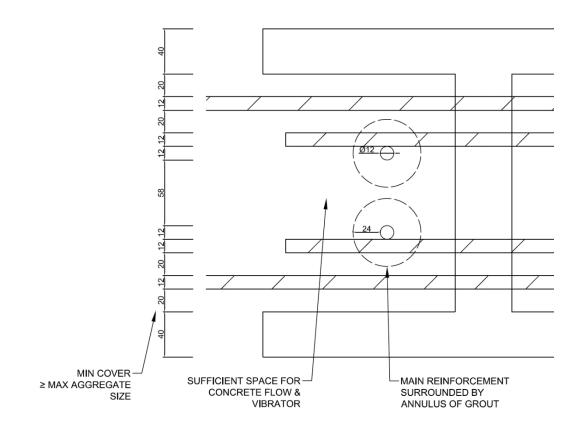
**Figure 4** – N12 Vertical and Horizontal Bars each face within a 30.48 'H' Block, at location where horizontal bars are spliced.
