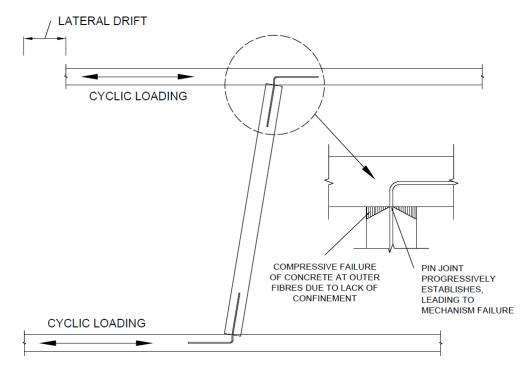
*Figure 1* – Idealised behaviour from walls with pin connection to slabs (central 'L' bars)
