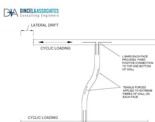
*Figure 2* – Idealised behaviour from walls with fixed connection to slabs ('L' bars to each face)
