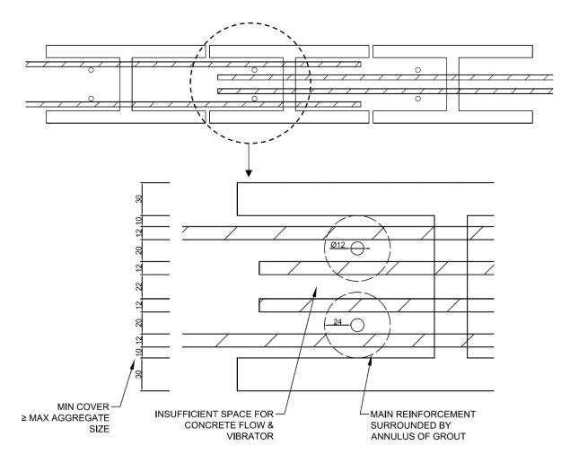
**Figure 3** – N12 Vertical and Horizontal Bars each face within a 20.48 'H' Block, at location where horizontal bars are spliced.
