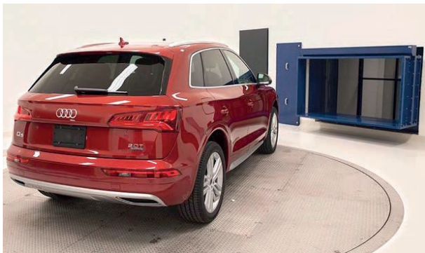
Fahrtwind-Simulator type VAF 3934, air outlet side rotating platform
