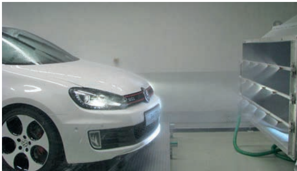
Simulation of rain using attached spray bars
