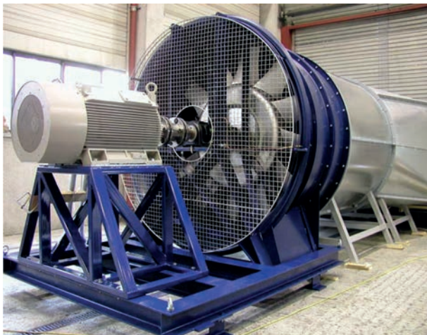
Fahrtwind-Simulator type VAF 2240 E3794, air intake side
