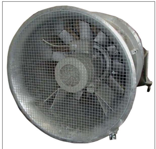
Fahrtwind-Simulator type VAF 1400 - air inlet side
