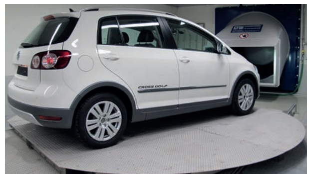
Fahrtwind-Simulator type VAF 2240, outlet side, turntable
