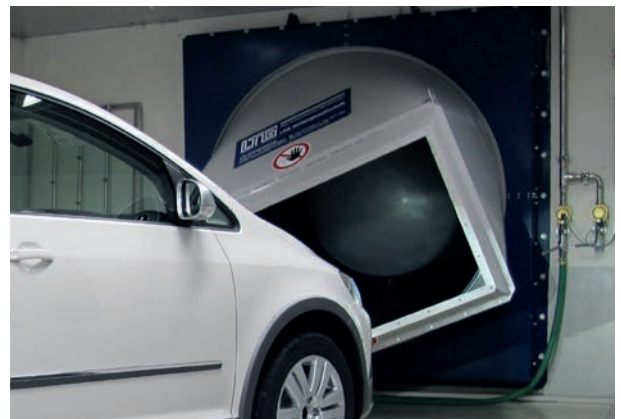
Fahrtwind-Simulator type VAF 2240 - outlet nozzle rotatable by 360°
