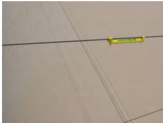
Figure 22. Line level on string.
