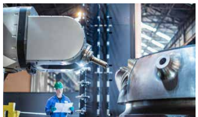
5-Axis Machining of an Ultra-Large Component
