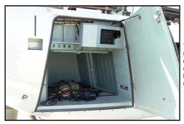
The luggage compartment is able to contain up to 5 large suitcases. When the helicopter is configured for internal freight transport, the cabin area plus luggage compartment make loading and unloading effortless thanks to an unobstructed cabin and a flat floor.
