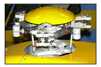
The main rotor generates the lift and the traction transferred to the helicopter. During flight, it allows the helicopter to be controlled in roll and pitch in conjunction with the tail rotor (yaw).
