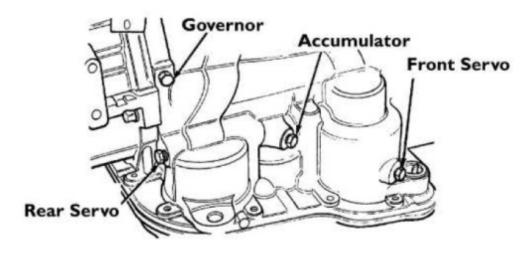
Use the accumulator and rear servo pressure ports to check main pressure with 0-300 p.s.i. gauge. (There is no specific Main line pressure tap) Apply the parking brake and block the wheels when testing.
