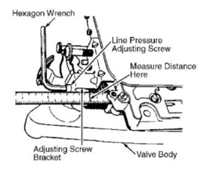
The Main pressure regulator valve is adjustable with an allen wrench with the oil pan off. The base adjustment is measured from the valve body casting to the bottom of the adjuster plate as seen in the above picture. The base measurement is
