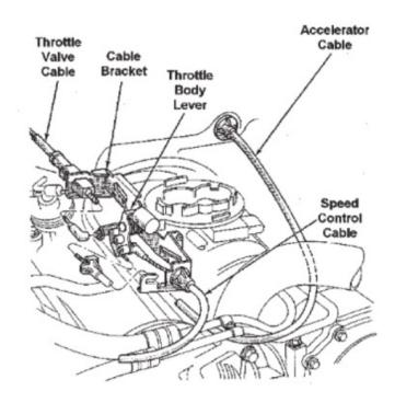
Sample of TV cable routing and adjustment at engine.
