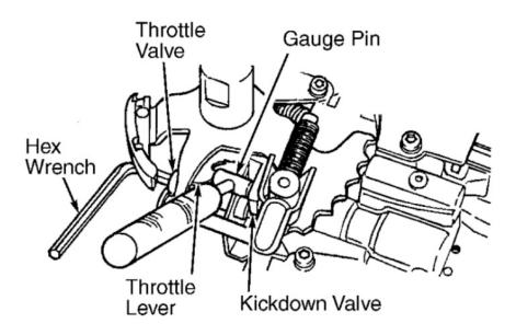
The TV has a base adjustment using tool # C-3763 which can be checked with pan off and adjusted with an allen wrench. If you don't have the tool you can make one or use small machinist's gauge block to check. Measurement should be: .627 inch.
