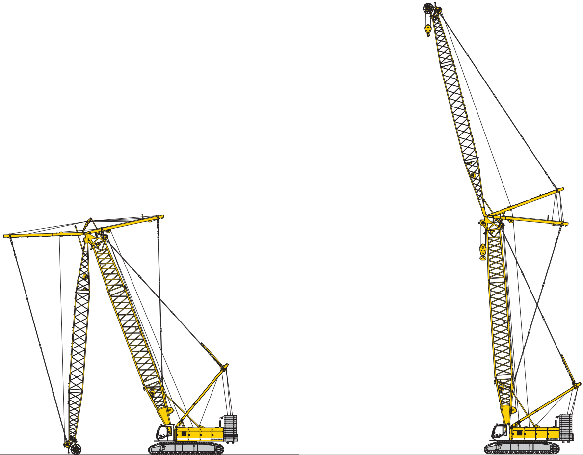
Erecting of main boom and luffing jib
