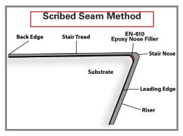
When butting stair tread and riser seams using the Scribed Seam Method, ensure that the stair tread above and below the riser, as well as the riser itself, have been trimmed and fit the step snuggly. Ensure the stair tread below the riser is in place prior to scribing the riser to ensure a tight fit to the leading edge of the stair tread above.
