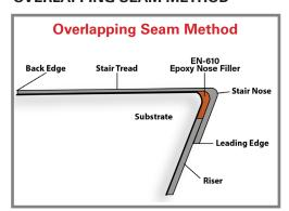
When overlapping stair tread and riser seams, ensure that the stair tread and riser have been trimmed and fit the step snuggly. Risers do not normally require trimming on the top edge prior to installation when overlapping seams. However, if the top edge of the riser extends up to or over the height of the
