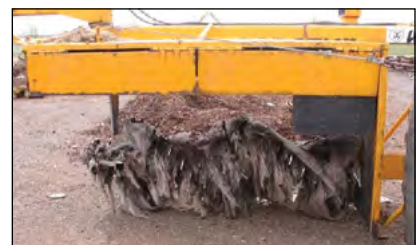
Photo 12-7: Bags and other plastic contamination can become tangled in windrow turners and are very difficult to remove © Scott Gamble
