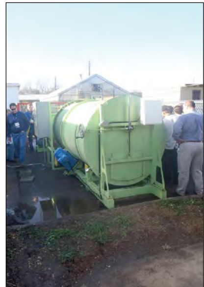
Photo 5-28: Small-scale rotating drum system © CH2M HILL
