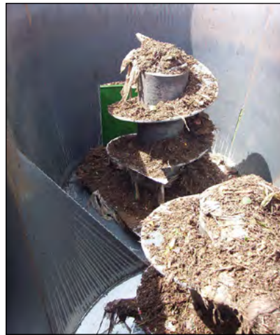
Photo 11-4: Augers inside a vertical mixer © Scott Gamble
