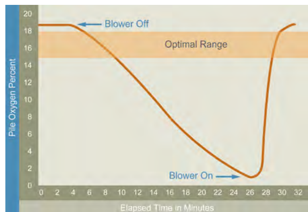
Figure 3-7: Decline of oxygen levels in an aerated composting pile. The concentration of oxygen in a compost pile can be consumed very rapidly during the active composting step.
