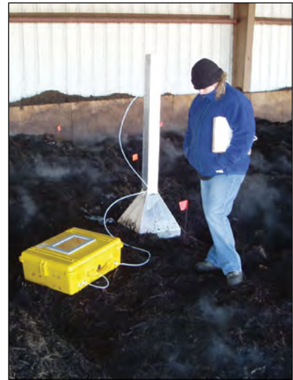
Photo 14-2: Sampling hood being used to collect odour samples from an aerated compost pile © CH2M HILL
