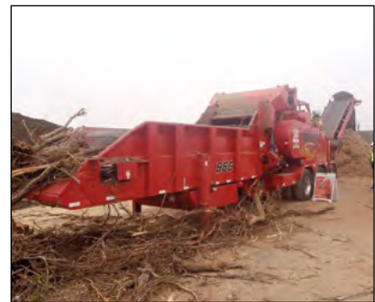
Photo 11-11: Horizontal grinder © CH2M HILL
