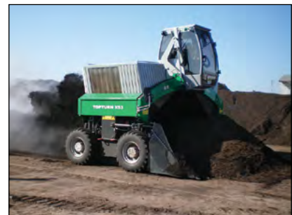
Photo 5-7: Straddle-style windrow turner © CH2M HILL
