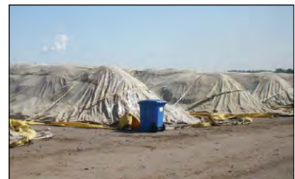
Photo 5-15: Covered, positively aerated composting system © CH2M HILL
