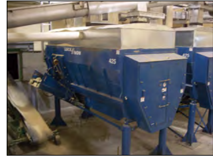
Photo 11-5: Horizontal auger mixer © CH2M HILL
