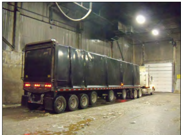
Photo 8-2: Using transfer stations and long-haul trailers can make hauling organics to distant facilities more economical © CH2M HILL
