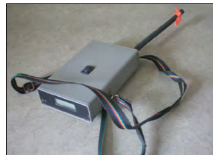
Photo 3-7: Specialized instruments are used to measure oxygen levels in compost piles © CH2M HILL
