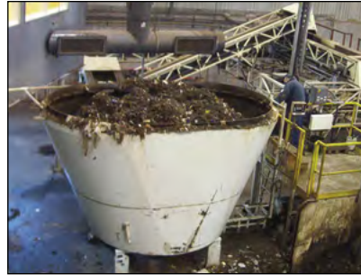
Photo 11-3: Vertical auger mixing unit © Scott Gamble
