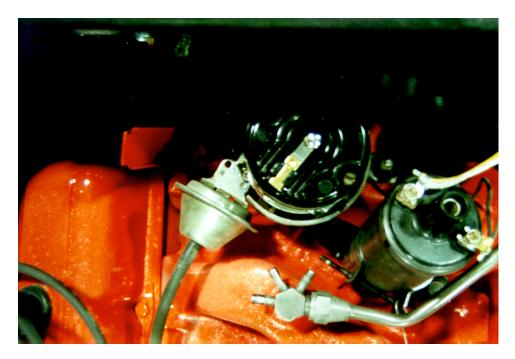
Figure 1: Distributor & Rotor Correctly Installed at #1 Firing Position
