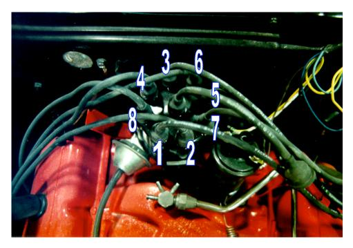
Figure 2: Correct Spark plug Wire Order and Placement
