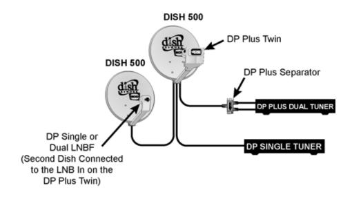
Figure 15. DISH Pro Plus Twin LNBF, DISH Pro LNBF, One DISH Pro Plus Separator, One DISH Pro Plus Receiver, and One DISH Pro Receiver
