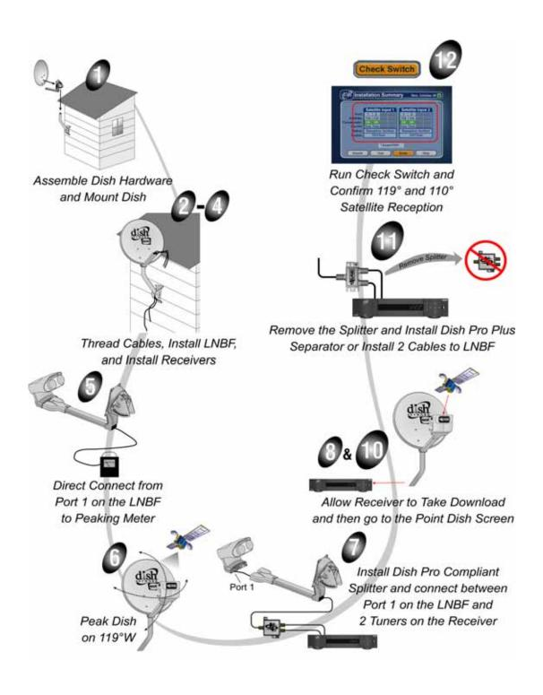
Figure 8. Installing the DISH Pro Plus Twin LNBF on any DISH Network Receiver
