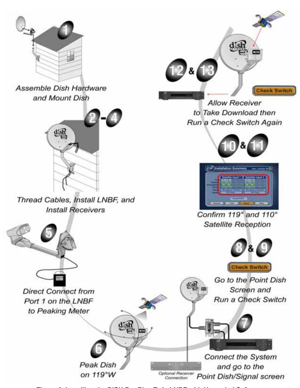
Figure 6. Installing the DISH Pro Plus Twin LNBF with Upgraded Software
