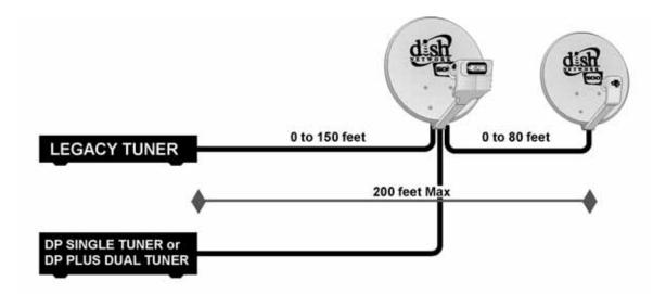
**Example**: If you have a Legacy receiver attached 150 feet from a DISH Pro Plus Twin and a Single LNBF 50 feet from the DPP Twin, then the DP or DP Plus receiver must be within 150 feet of the DPP Twin. The cable length between the DPP Twin and the Single LNBF is limited to 50 feet because the maximum distance between the Legacy receiver and the Single LNBF is 200 feet.
