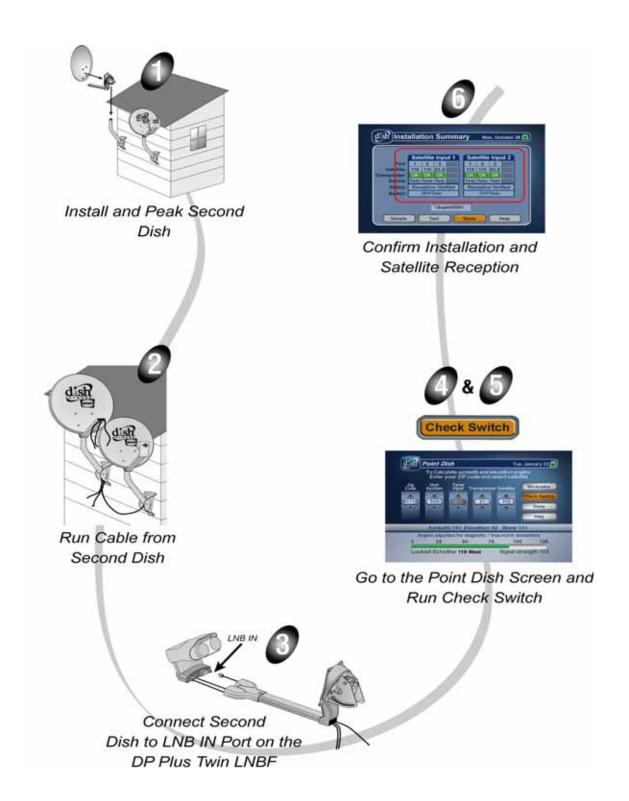
Figure 11. Connecting a Second Satellite Dish
