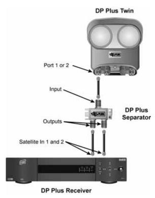
Figure 14. DISH Pro Plus Twin LNBF, DISH Pro Plus Separator, and a DISH Pro Plus Receiver
