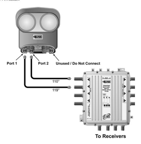
Figure 12. Connecting to a DISH Pro Plus 44 Switch
