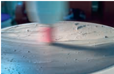
Computer controlled lapping (CCL) is the highly abrasive process step for coarse figuring.
