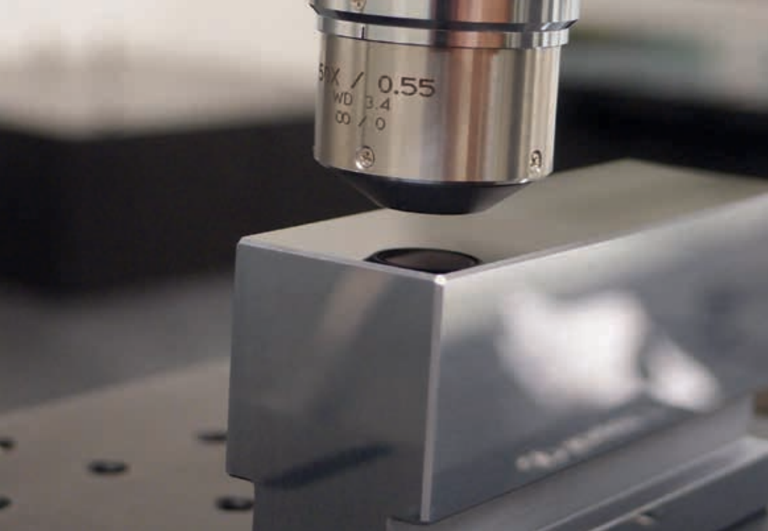
Mid-spatial frequency roughness (MSFR) detected with microinterferometry (ZYGO NewView 700).
