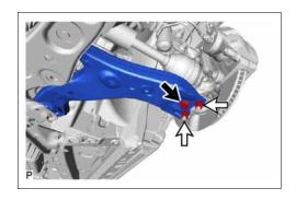
c. Connect the front lower No. 1 suspension arm subassembly to the front lower ball joint assembly with the bolt and 2 nuts.
