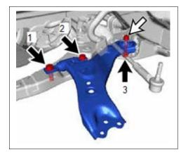
b. Install the front lower No. 1 suspension arm subassembly to the front frame assembly with the 3 bolts and nut in the order shown in the illustration.
