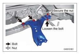
b. Remove the 3 bolts, nut and front lower No. 1 suspension arm sub-assembly from the front frame assembly.
