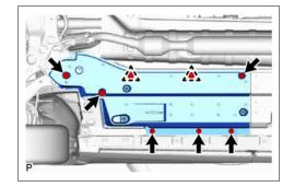
b. Attach the 2 clips and install the 2 bolts and 4 screws.
