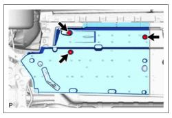
b. Loosen the 3 nuts and remove the front floor cover LH from the body.
