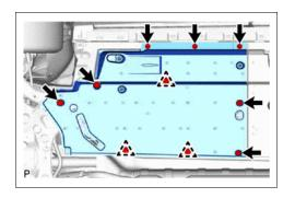
b. Attach the 3 clips and install the 2 bolts and 5 screws.
