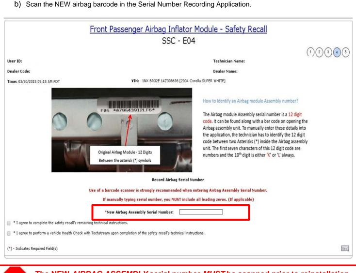
The NEW AIRBAG ASSEMBLY serial number MUST be scanned prior to reinstallation to track the airbag assembly to the vehicle.
