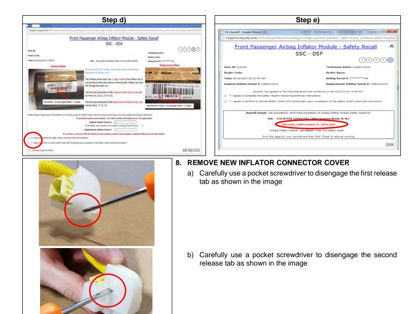
c) Open the connector cover. Once open carefully use a pocket screwdriver to disengage the release tab and remove the connector cover from the connector
